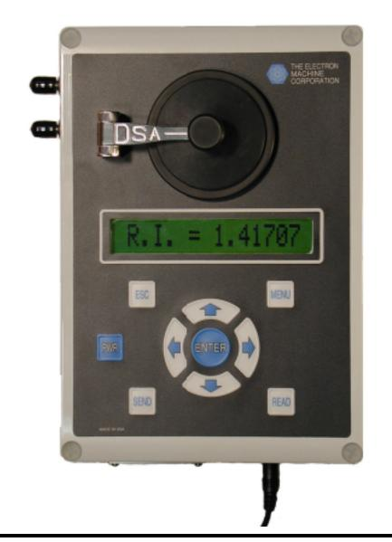
The DSA E-Scan is an automatic, benchtop critical angle refractometer with a digital readout and temperature-controlled sample chamber. It measures the critical angle of refraction of sample fluids which are directly correlated to various measurements including percent dissolved solids, Brix, and refractive index. The instrument is equipped with a menu-driven user interface and is factory calibrated and temperature compensated.
