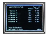
9. Edit console "Volts" to match EOS sheet provided with replacement sensing head. Start with Sample 1 (To edit console "volts" values. LEFT arrow to highlight "volts". Key in EOS values for highlighted sample. Push ENTER.). \* Step 10A for Non-Color MPR \*\* Step 10B for Color MPR Doors \*\*\* Step 10C for MDS Refractometer
